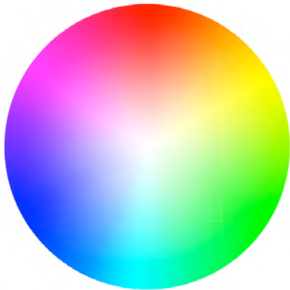
Fig. 4.3: a colour wheel. Along its edge are the fully saturated colours. Towards to the middle of the wheel the colours desaturate. White is at the centre.
